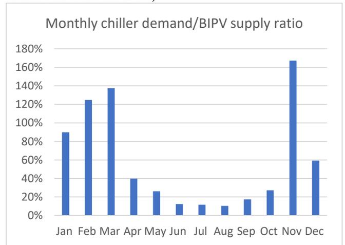
Figure 9. Monthly chiller demand/BIPV supply ratio
