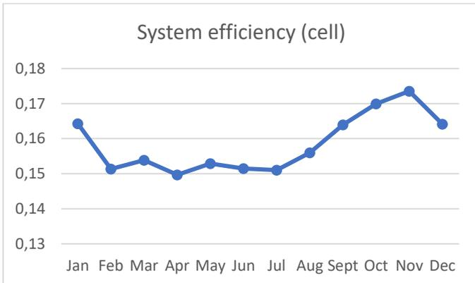
Figure 7. Monthly system (cell) efficiency - experimental
